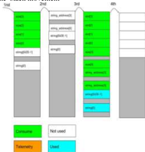
Figure 4.2: Stack variation per command executed
